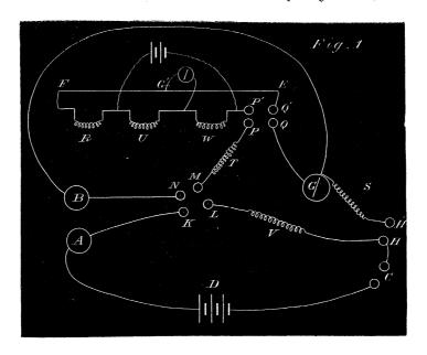
P, Q, H, and H' are also mercury cups. C is the commutator, and D the battery. Between H' and G is a resistance, S, of about 3000 B.A. units, between H and L a second resistance, V, of about 1 unit.
