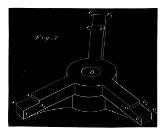
To place the second coil with its plane parallel to the first we used three cylinders of brass, the ends of which had been carefully turned so as to be at right angles to their axes, while the lengths of the cylinders were as nearly as possible the same.
